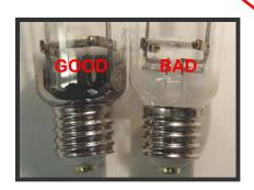
Getter Flash absorbs oxygen, hydrogen and other impurities present within the lamp. These impurities can result in the rapid deterioration of the metal parts...resulting in lamp failure
